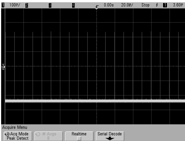
Figure 48 15 ns Narrow Pulse, 20 ns/div, Peak Detect Mode
